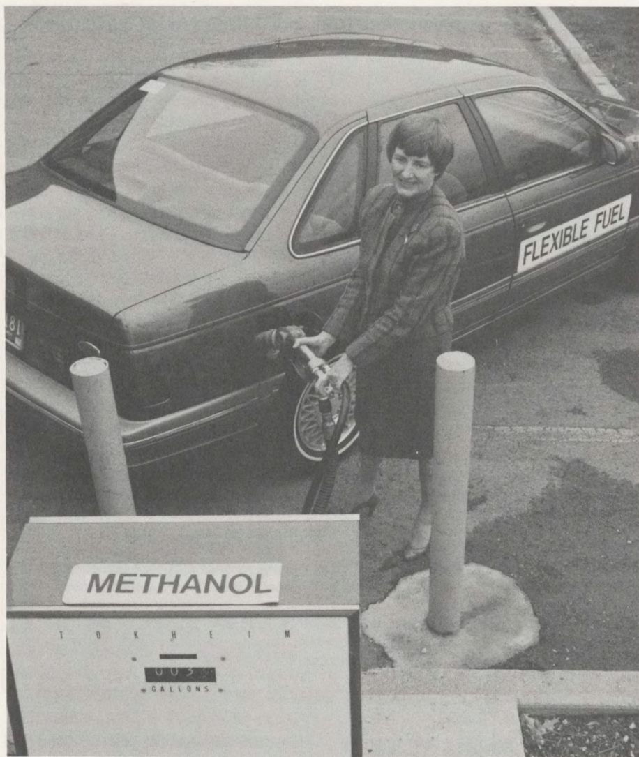
U.S. auto companies have modified regular production models to run on methanol, ethanol, gasoline, or any combination of these fuels.
