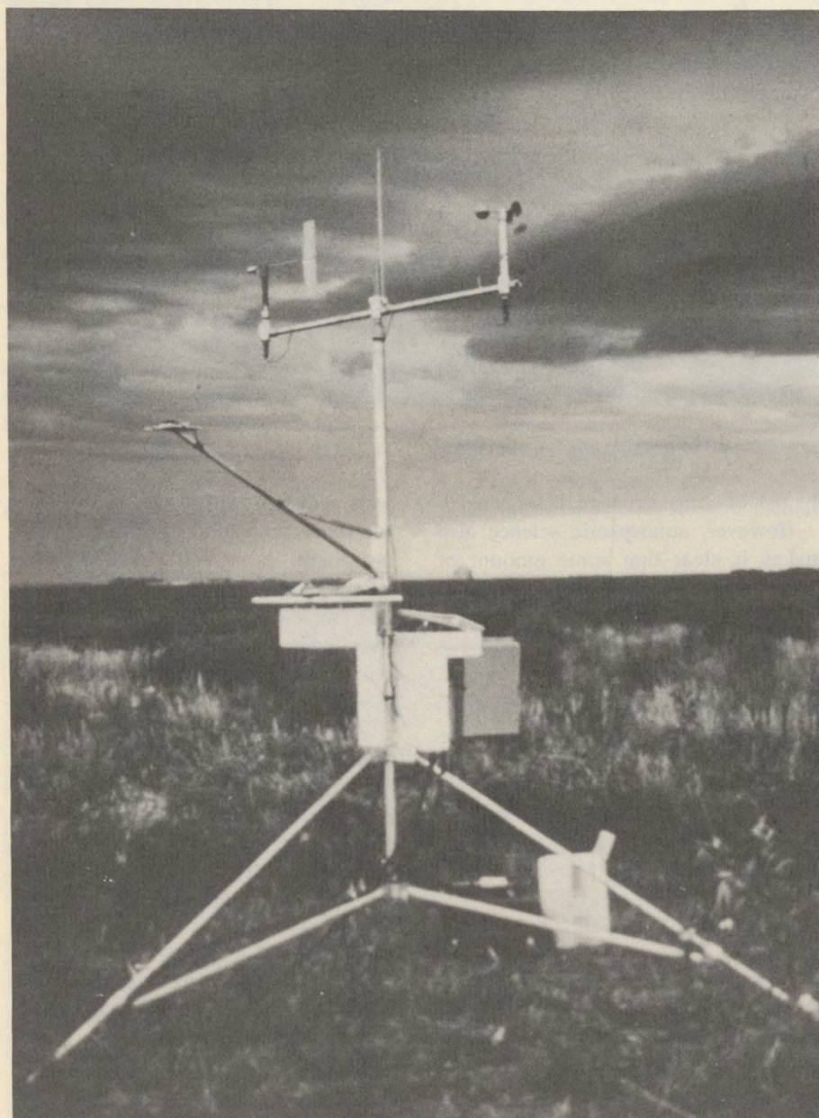
Technical advances like this automatic weather station, which guides irrigation scheduling, could help save water when supplies are short, as they may be if the climate changes.
